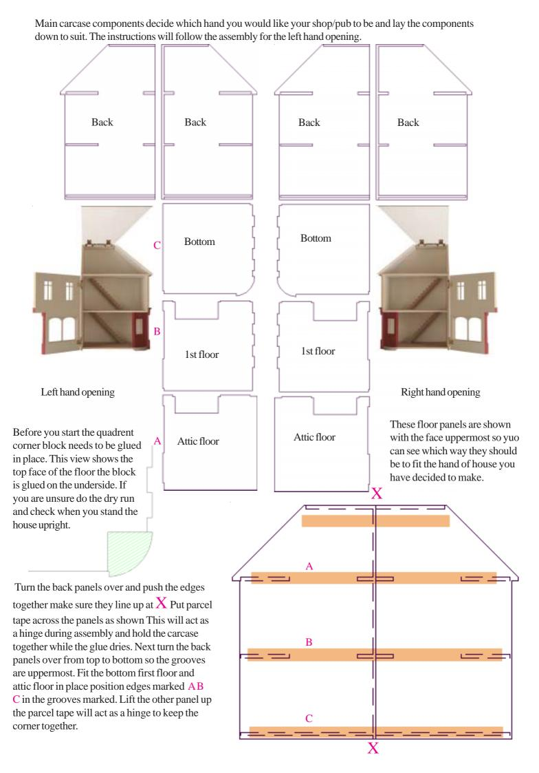
Stand the house up and put parcel tape on as shown. Stick the tape firmly on the edge top and bottom of the floor and pull tight around and onto the back panel. do this to all three floors. Make sure all floors are pushed right back into the grooves before leaving it for the glue to dry.
