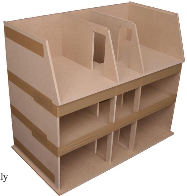
Make sure the carcass is standing level and is undisturbed until the glue is fully dry. Any movement after it has started setting but before the glue is dry will cause a permanent fault in the glue joint
